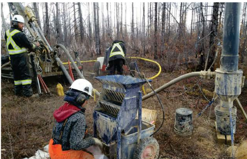
RAB drill operating on the Mariposa property, September 2015.
